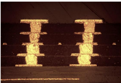
Scan shows 4 stacks of microvias and the adjoining finely etched traces
