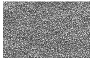
Ultra Low Profile Copper (Treated surface) x 3,000
